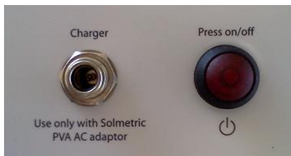
Figure 11. Battery charger connector on the PVA-600
