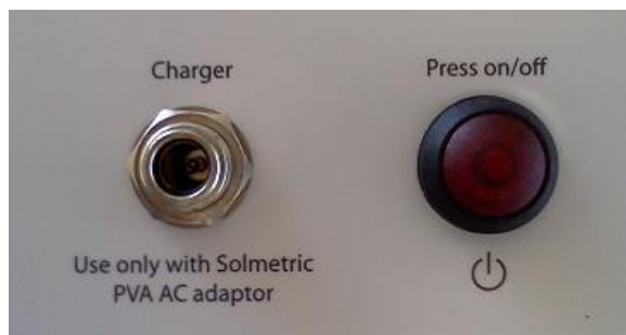
Figure 18. Powering-up the I-V Measurement Unit
