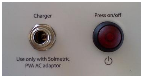
Figure 44. Turn on the I-V Measurement Unit
