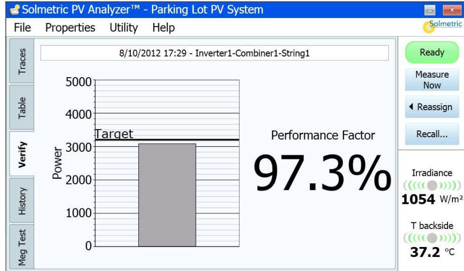
Figure 49. Verify tab with maximum power indicator and Performance Factor
