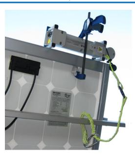
Figure 18. SolSensor tool lanyard secured to a racking member.
