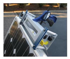
Figure 17. SolSensor mounted on the frame of a PV module
