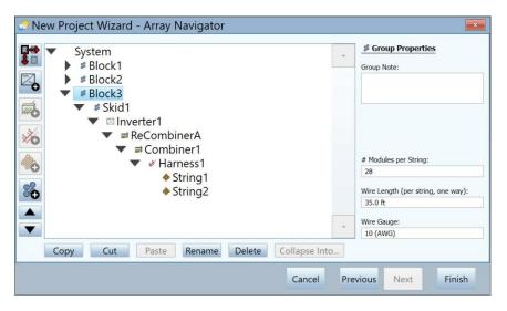
Figure 36. Finished array tree for a utility PV field.
