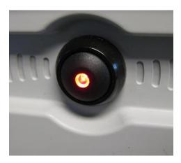
Figure 23. SolSensor pushbutton with LED lit. LED blinks until wireless network is established, after which it remains on.
